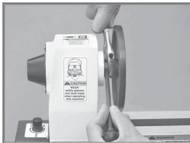
Figure 11. Tightening face plate to headstock spindle.
