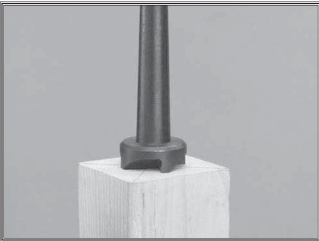
Figure 1. Center fully embedded in workpiece.
