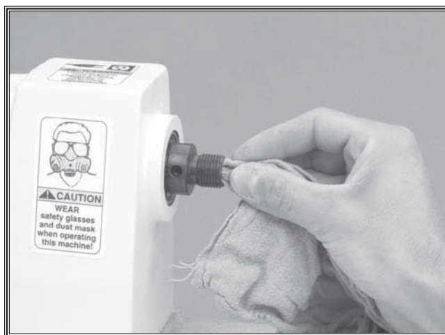
Figure 32. Cleaning spindle tapers.
