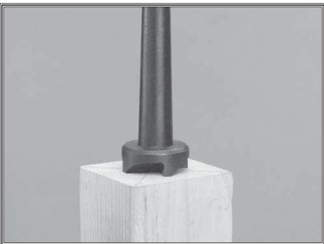
Figure 25. Spur center properly embedded into workpiece.
