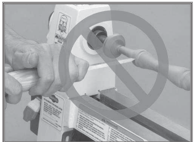
Figure 6. DO NOT cut without using tool rest.
