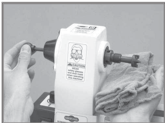
Figure 10. Removing spur center with knock-out tool.
