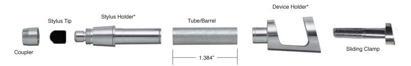
\*Do not press directly on Stylus Holder or Device Holder. See Diagram C
